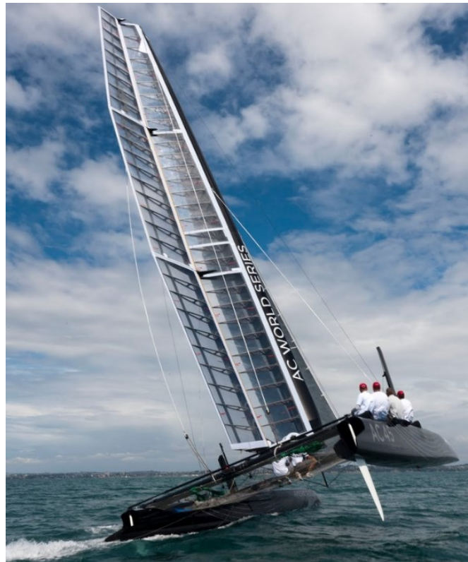
Figure 7 Rigid sail on an AC45 (10)
