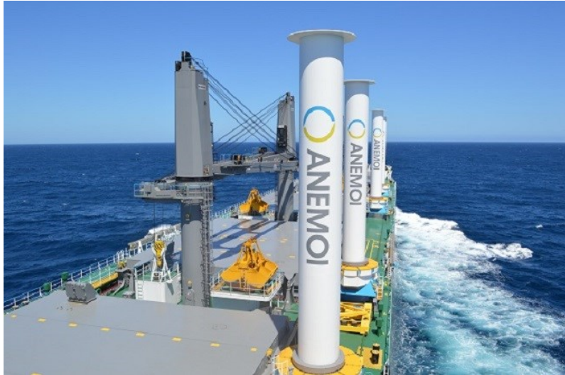
Figure 5 Flettner Rotors in action (8)
