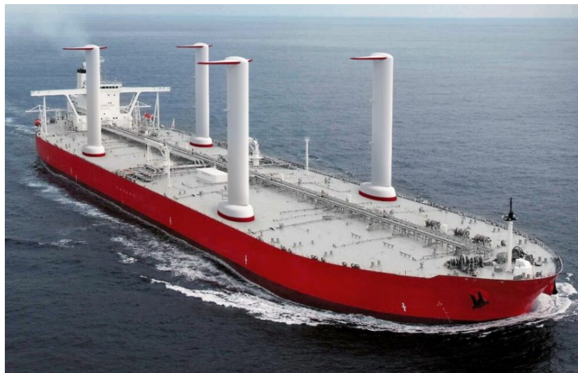
Figure 6 Suction wings application (9)
