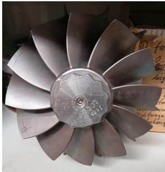
Figure 3.3: Axial view of the turbine impeller, dismantled
