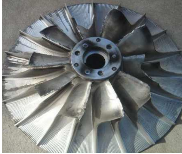
Figure 1.1: Example of crack fatigue overwhelmed impeller [2]
