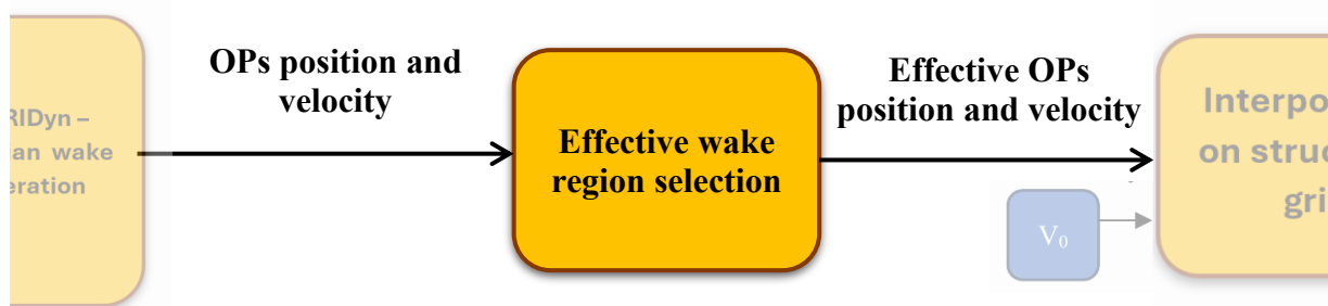
Figure 22 - input/output of the "Effective wake region selection" block. It is the first one of wake processing chain
