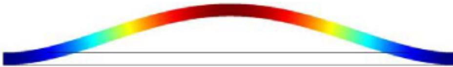
Figura 9 Modo di vibrare Clamped-Clamped beam (Guoqiang Wu, 2020)
