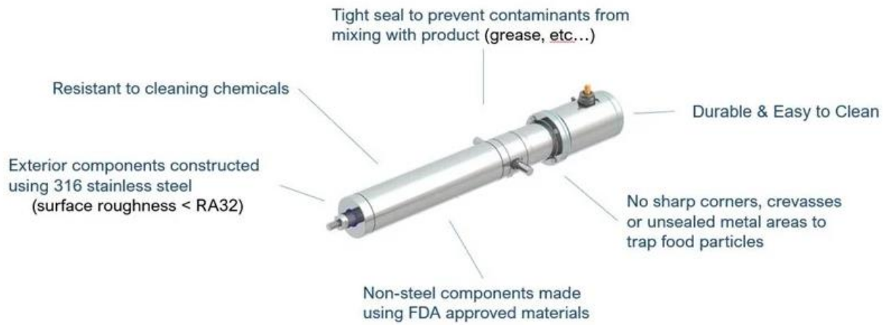
Fig. 3.7: An example of Food and Beverage grade hydraulic actuator
