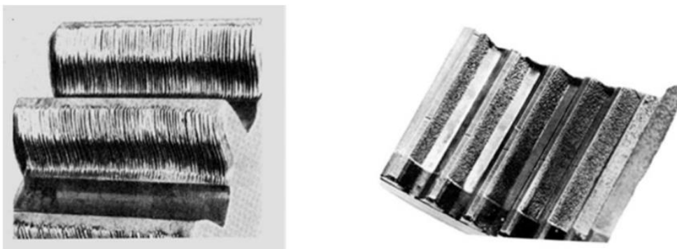
Figure 2.8: Wear corrosion induced by chemical reactions in the lubricating oil
