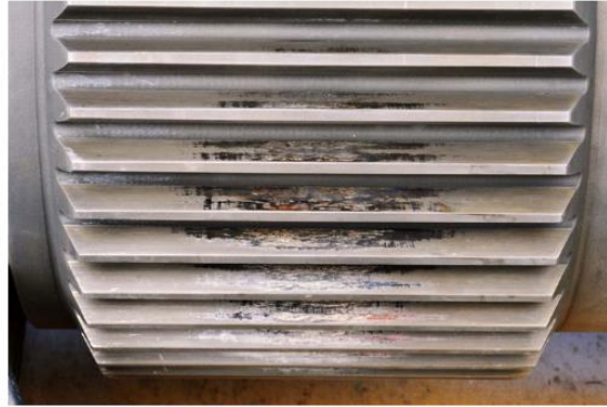
Figure 2.11: Severe fretting corrosion on a gear tooth
