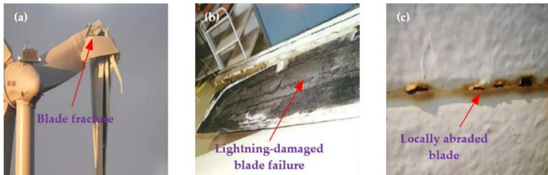
Figure 2.7: Real images of wind turbine blades affected by different types of failure: structural fracture, lightning damage, and surface abrasion
