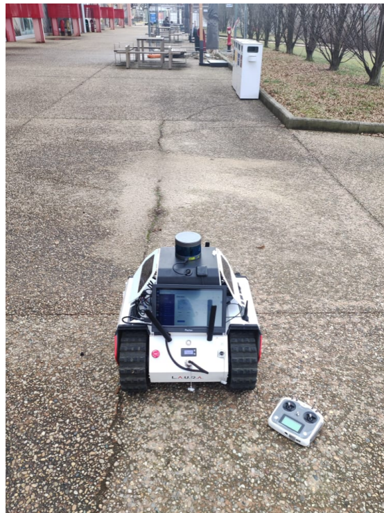
Figure 5.19: HIL Implementation of the AgileX Bunker Mini robot in the outdoor environment.
