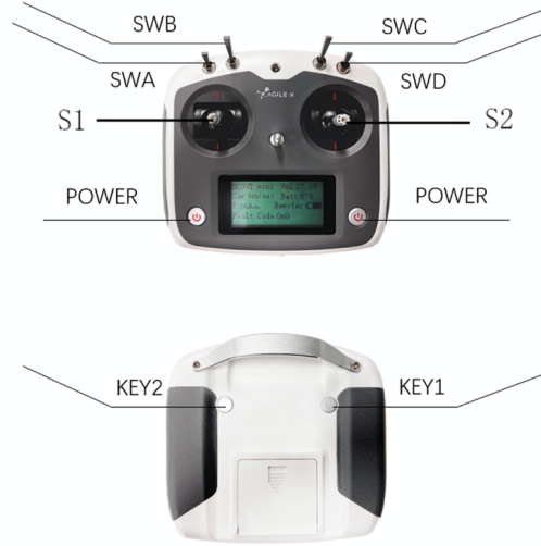
Figure 4.5: Schematic Diagram of the Remote Controller for Manual Teleoperation.
