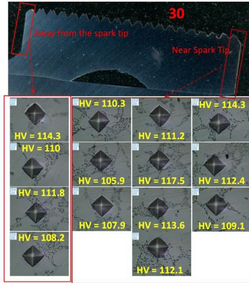
Figure 43. Engine head specimen and result from the microhardness test in different sites.
