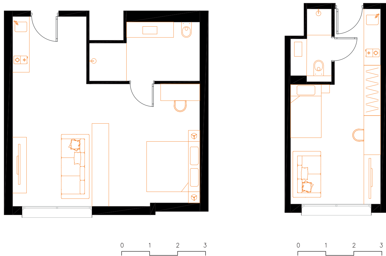
Figure 46- The plans illustrate two compact micro-unit layouts used within the residential block: Type 1 (single compact unit) and Type 2 (extended double-use model). Drawn by the author based on original architectural documentation.
