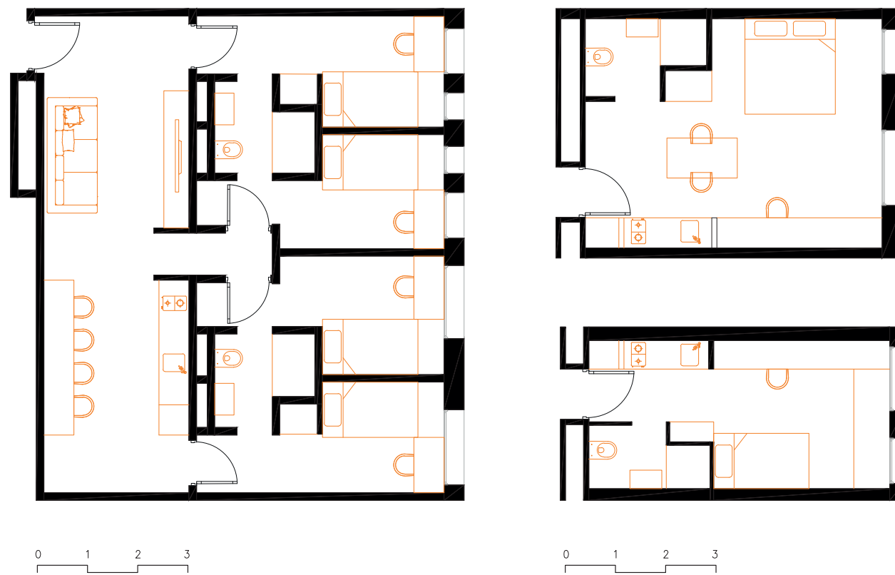
Figure 55- The plans illustrate three micro-unit typologies implemented within the residential block: Type 1 (single compact unit), Type 2 (extended double-use unit), and Type 3 (linear studio with separated functions). Drawn by the author based on original architectural documentation.
