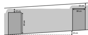
Figure 21. Schematic representation of the water flow in the channel at the center of Perge main street/ Debaste, F., & Haut, B. (2014). Some elements of the water supply system of the city of Perge, in the Roman Imperial period, IWA Regional Symposium
