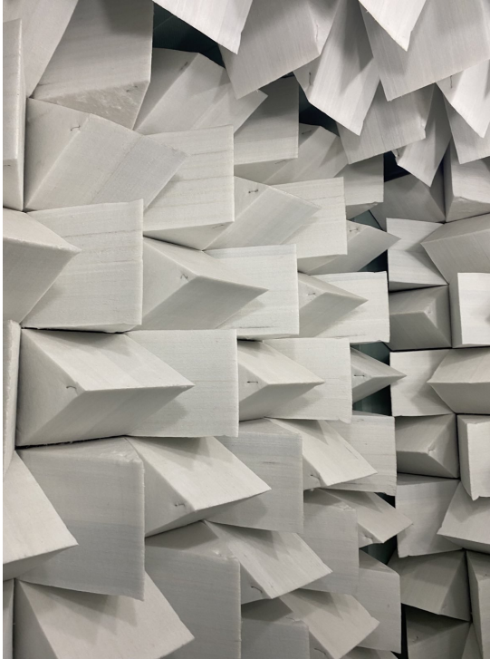
Figure 5.22: The walls covered with sound-absorbing materials at the anechoic chamber of the Politecnico di Torino.
