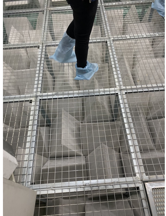
Figure 5.23: The suspended mesh on the floor at the anechoic chamber of the Politecnico di Torino.
