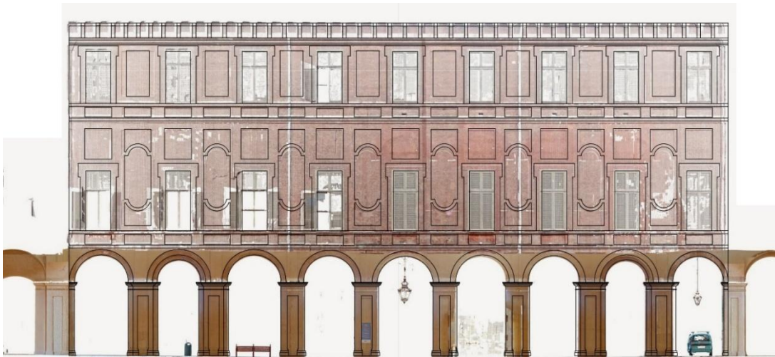
Figure 6.8. Courtyard LOG modeling. Detailed HBIM representation of the Courtyard façade at LOG 400, showing accurate modeling of arches, cornices, and column bases derived from point cloud data. The geometric fully reflects advanced parametric design practices in Revit for heritage modeling.
