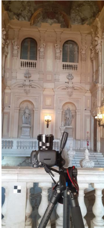
Figure 5.3. Manual photogrammetry data acquisition using a digital camera and coded targets for ground control referencing and scaling. This procedure ensures accurate alignment and metric reliability of the 3D reconstruction. (Spanò et al., 2024)
