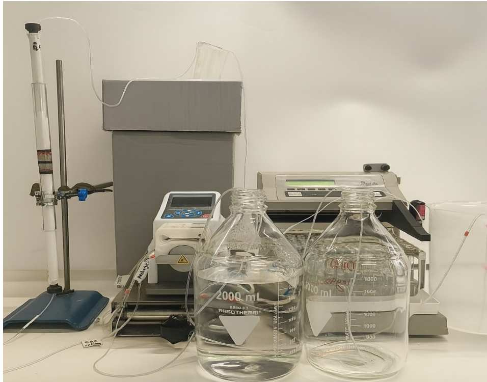
Figure 15. PFAS transport test-setup configuration
