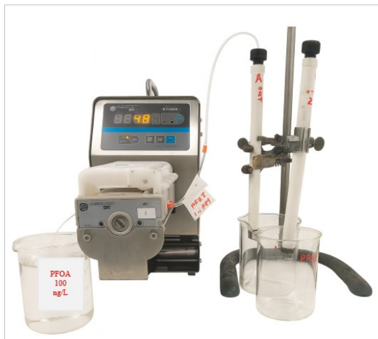
Figure 13. Configuration used for PFOA adsorption test
