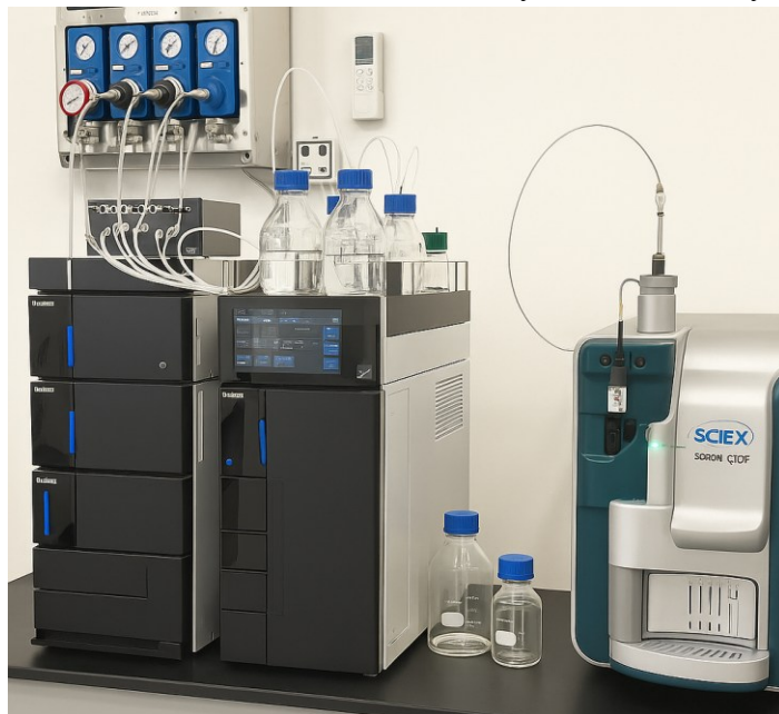
Figure 12. UHPLC system coupled with a QTOF mass spectrometer used for PFAS analysis
