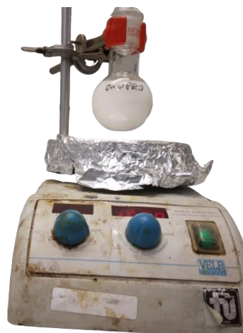
Figure 4: Magnetic stirrer for stirring, producing mixture of [Cho][Pro].
