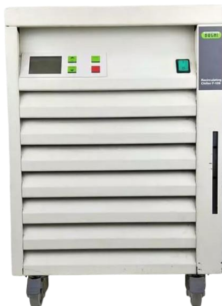
Figure 6: Chiller for producing below zero temperature for distillation of solvent.
