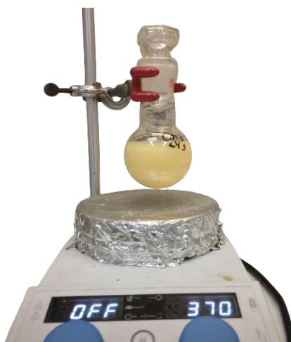
Figure 8: Device for stirring, producing mixture of [Cho][Lys].
