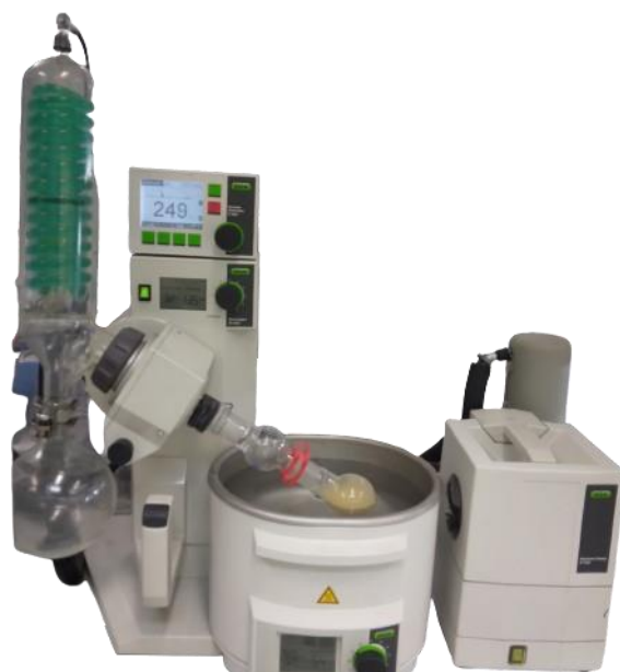
Figure 5: Rotary evaporator for heating [Cho][Pro], [Cho][Lys] and distillation of solvent.
