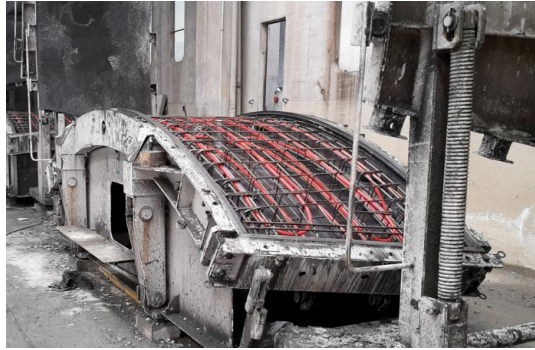
Figure 2-19. Absorber pipes of Enertun lining attached to the reinforcement cage during molding process (Barla et al., 2019)
