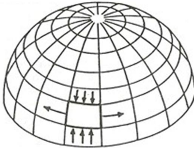
Figure 82 : Parallels in the domes require tensile strenght (Giuffrè, 1989).
