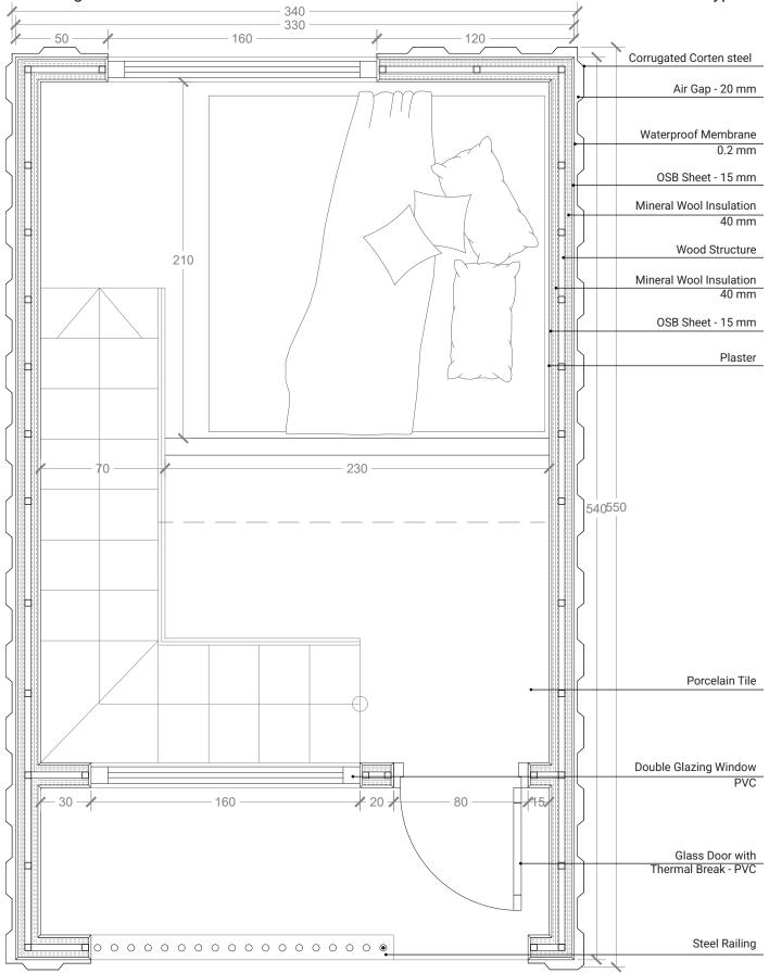
fig. 50- Intervention: Room Type 2, Bedroom for Families, 1st Floor Plan - Annotation in cm
