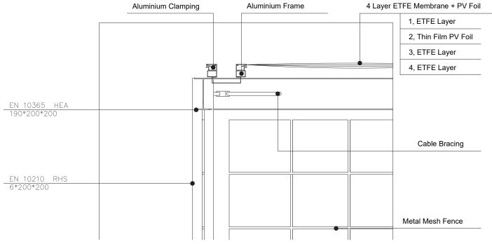
fig. 69- Roof Details and Materials
