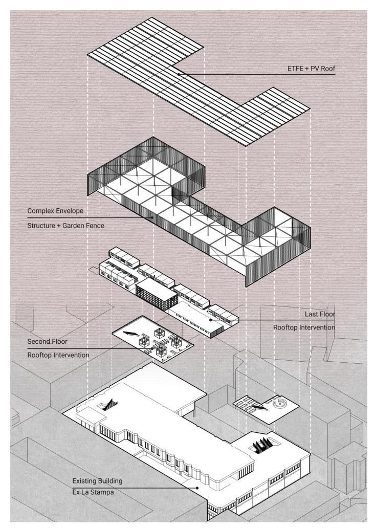
fig. 37- Exploded Axonometry Of The Intervention
