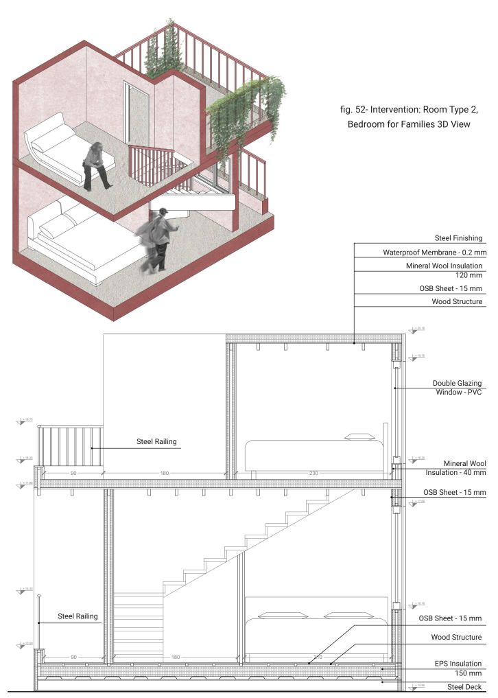
fig. 53- Intervention: Room Type 2, Bedroom for Families, 2nd Floor Section - Annotation in cm, Height in meters
