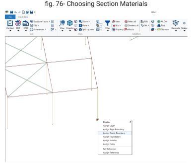
fig. 77- Adding Rigid Boundry to Each Column
