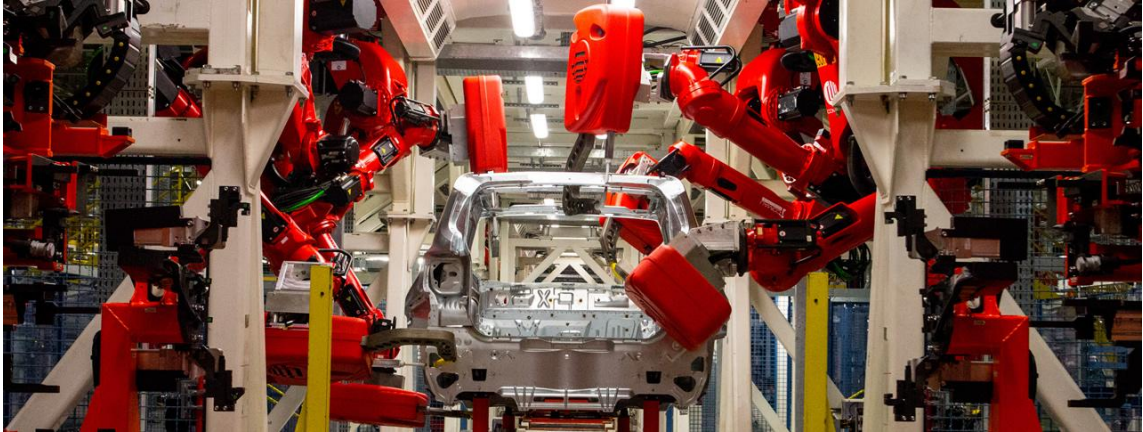
Figure 2.3: Comau robots of the NJ series working on a welding task. [7]
