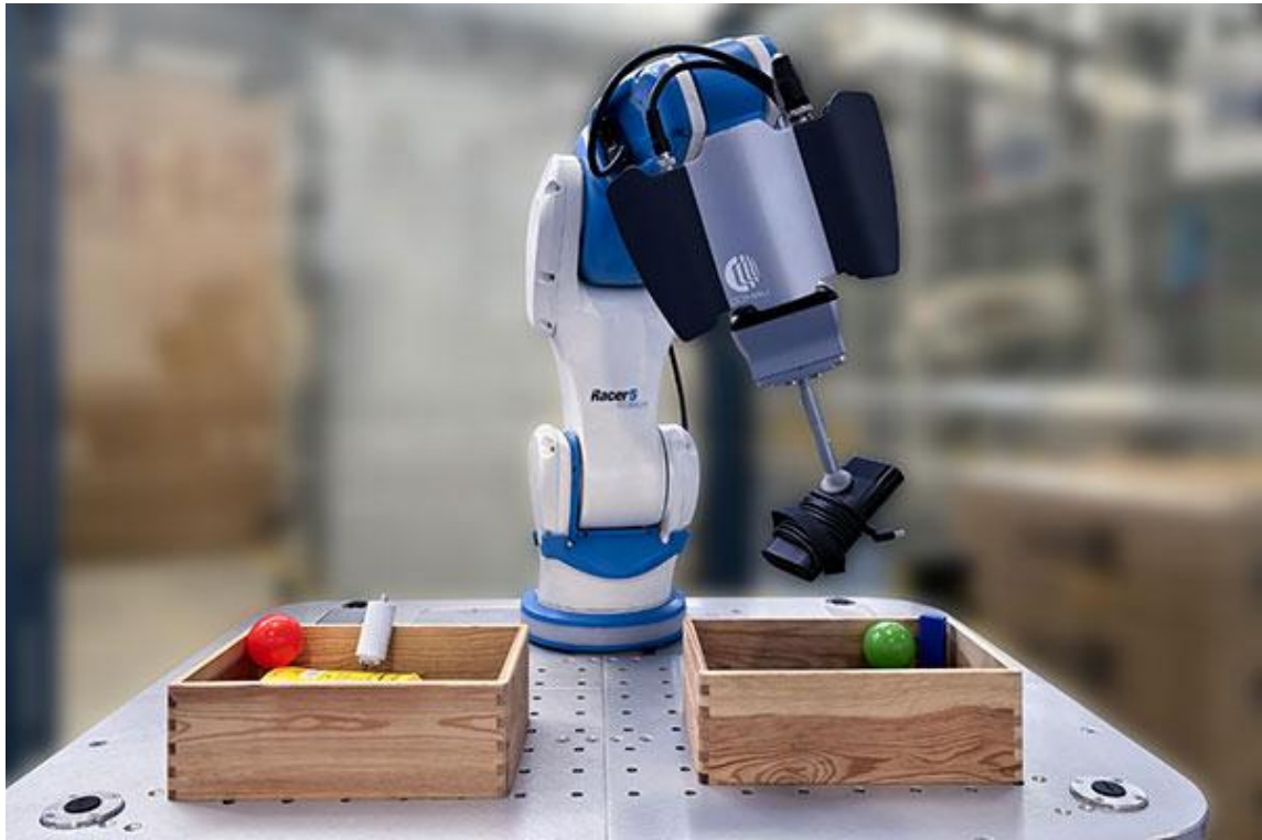
Figure 2.2: A Racers5-Cobot performing a pick and place operation [7]
