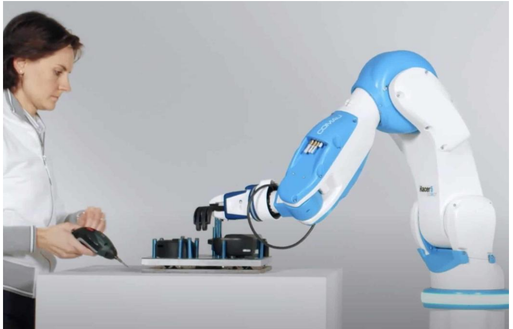
Figure 1.1: A comau racer5-cobot working alongside a human
