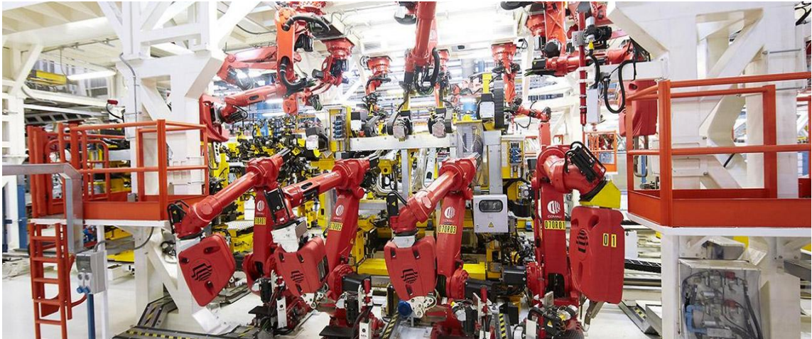
Figure 2.4: An assembly line made of Comau NJ Robots [7]
