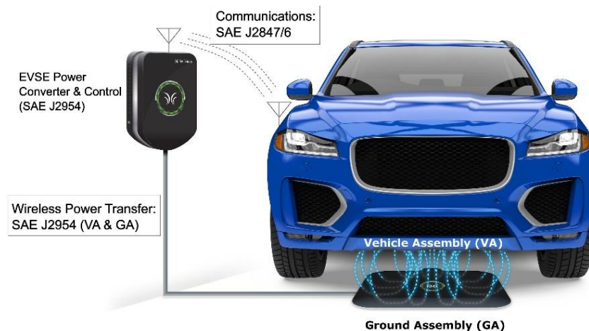
Figure 2: WPT for charging vehicle
