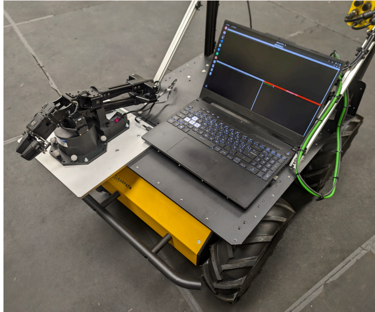
Figure 16: Integrated loco-manipulation system: WidowX 250 S, Husky A200, and offboard computer.
