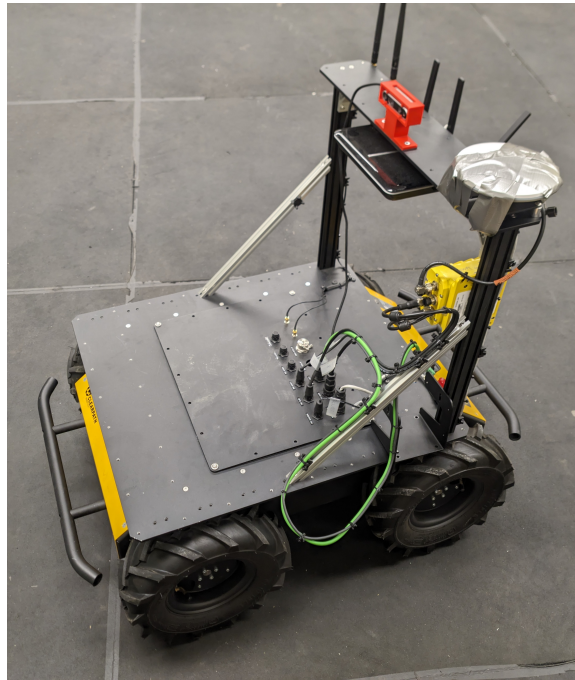
Figure 15: Clearpath Husky A200 UGV supporting the WidowX manipulator and computing platform.
