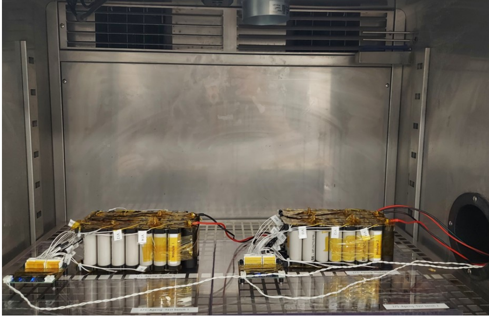
Figure 4.2: BALF's test bench lithium-ion battery packs connected to the slave boards
