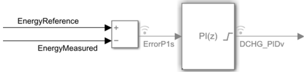
Figure 2.12: The discrete PI controller implemented in Simulink
