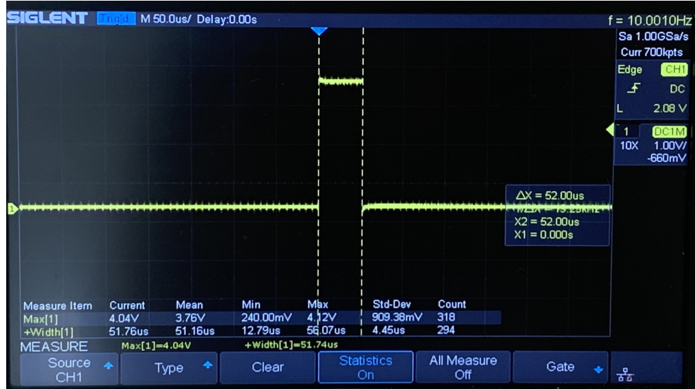
Figure 6.6: Oscilloscope displays the pulse width indicating the algorithm’s execution time
