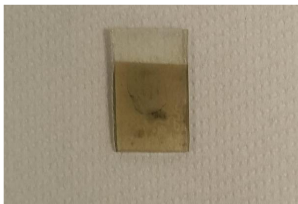
Figure 3b: MoS 2 film after ultrasonic spray coating (200 °C, 20L, 60S)
