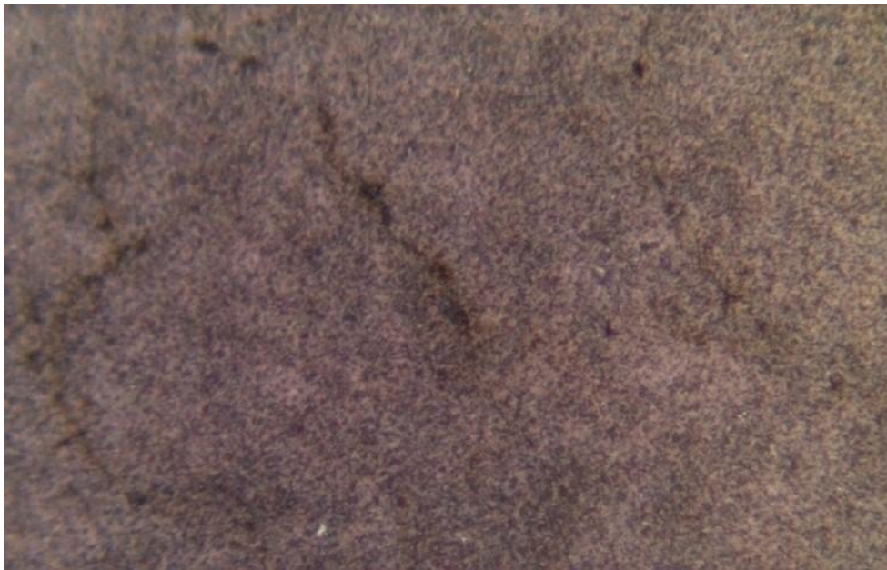
Figure 6: Optical micrograph of MoS 2 thin film (150 °C, 50L, 30S)
