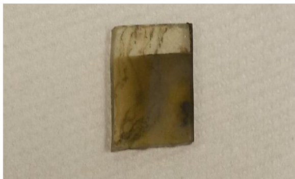
Figure 3d: MoS 2 film after ultrasonic spray coating (150 °C, 50L, 30S)
