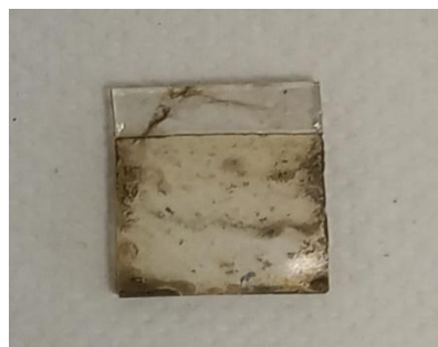
Figure 9e: WS 2 film after ultrasonic spray coating (200°C, 50L, 30S)
