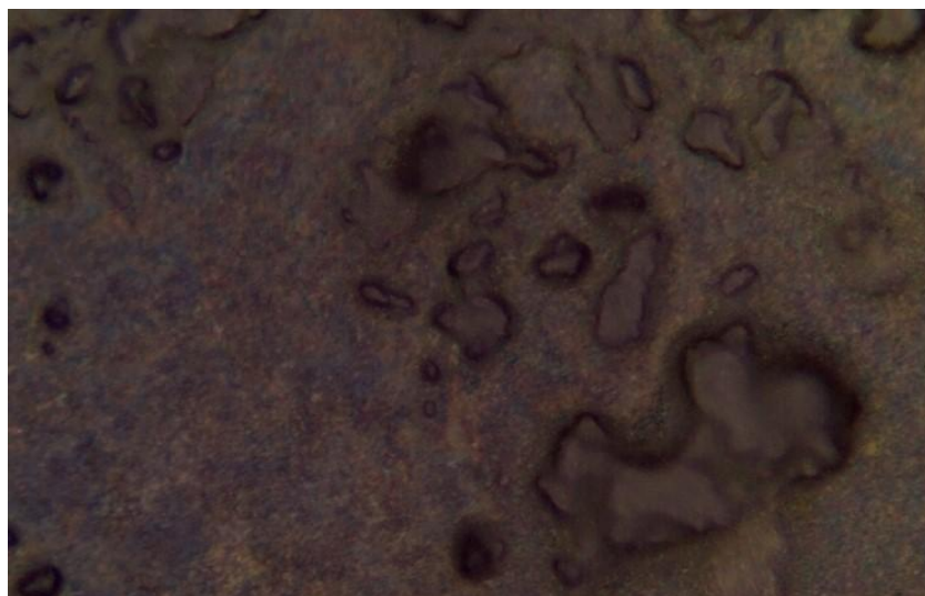
Figure 12: Optical micrograph of WS 2 thin film (150 °C, 20L, 60S)
