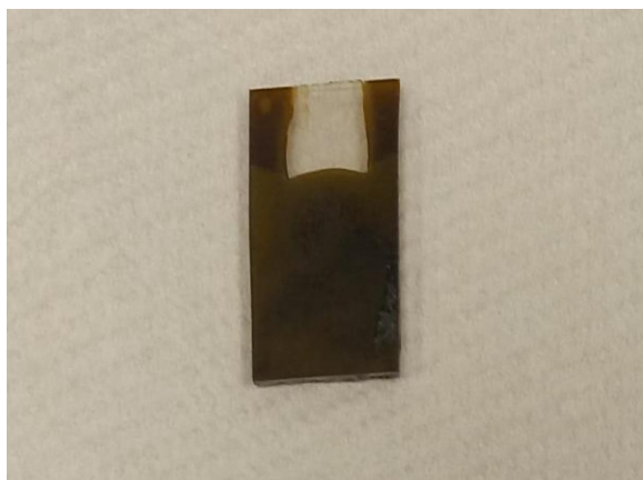
Figure 3e: MoS 2 film after ultrasonic spray coating (200 °C, 50L, 30S)
