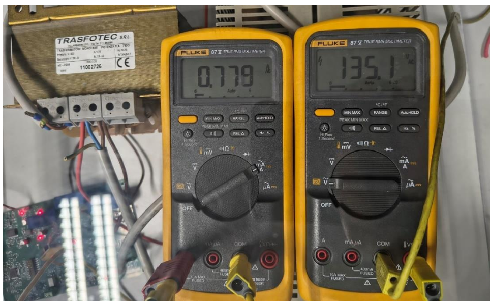
Figure 49 :Voltage and Current of Transformer and Rheostat
