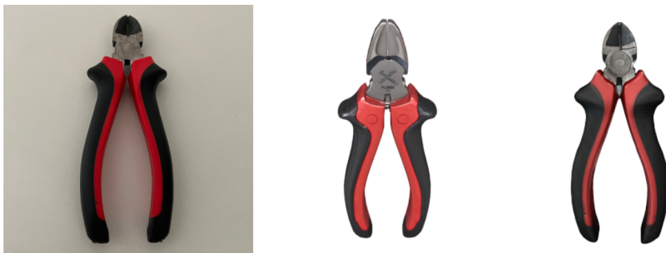
Figure 3.3: Comparison between the real wire cutter (left), the model generated with Meshy (center), and the model generated with StepFun (right).
