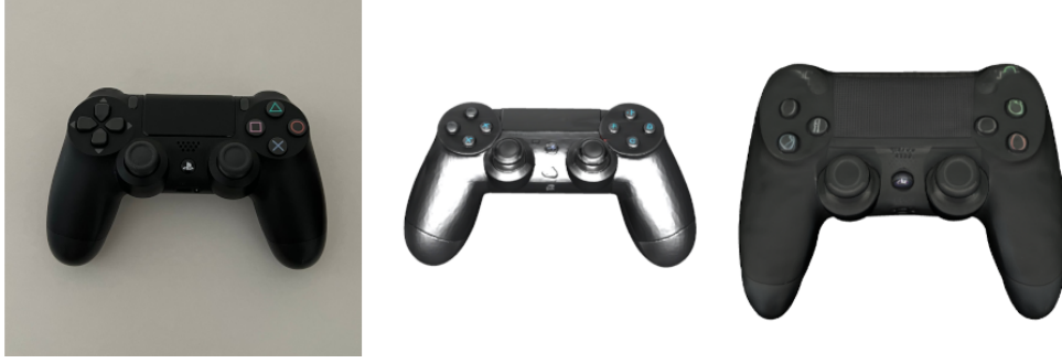
Figure 3.4: Comparison between the real joystick (left), the model generated with Meshy (center), and the model generated with StepFun (right).
