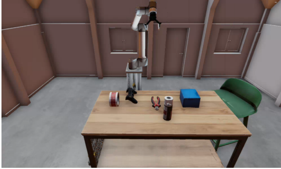
Figure 4.2: Simulated workspace in O3DE, showing the UR10e robot positioned on a desk and surrounded by AI-generated objects such as a joystick, spray can, and tape roll.
