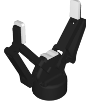
Figure 2.7: Robotiq 2F-140 adaptive gripper. Two-finger design with a 140 mm stroke, suitable for diverse object sizes.
