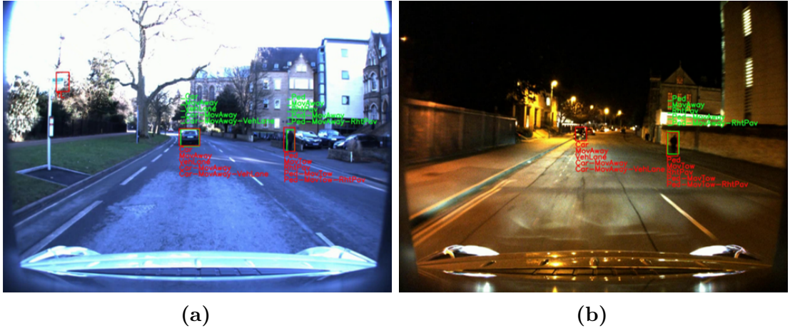
Figure 2.15: Two examples of frames sharing the same perspective but exhibiting different lighting conditions: (a) daytime image, (b) nighttime image. The Road Event annotations, as previously described, are highlighted, comparing the ground truth shown in green and the 3D-RetinaNet predictions in red.
