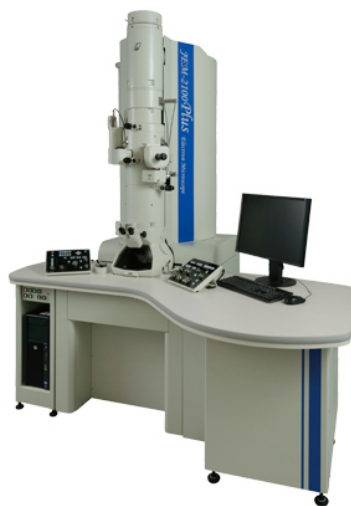
Figure 4: JEOL JEM-2100 transmission electron microscope used for nanoparticle imaging and morphological analysis. The instrument was operated to acquire TEM images for evaluating size, shape, and aspect ratio of the synthesized nanoparticles.
