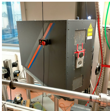
(b) KrF excimer laser (248 nm), model COMPex PRO 102 F by Coherent GmbH, used as the light source for all experiments.
