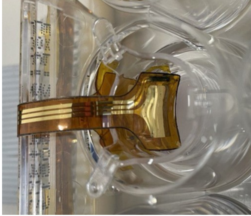
Figure 4.11: OECT mounted on the multiwell plate once the PEDOT:PSS channel is deposited.
