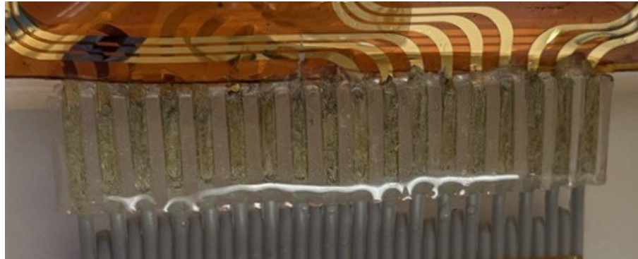
Figure 4.19: Close-up view of the passivation of the contacts. The resin endows the device with mechanical stability.
