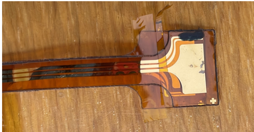
Figure 4.10: PEDOT:PSS channel deposited through drop-casting.
