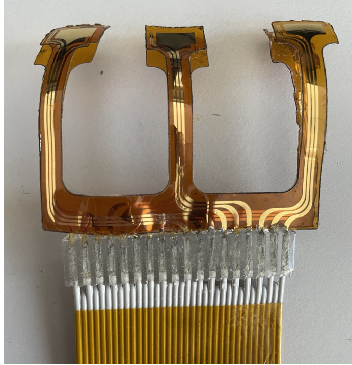
Figure 4.18: Image of the device after the contacts are passivated.
