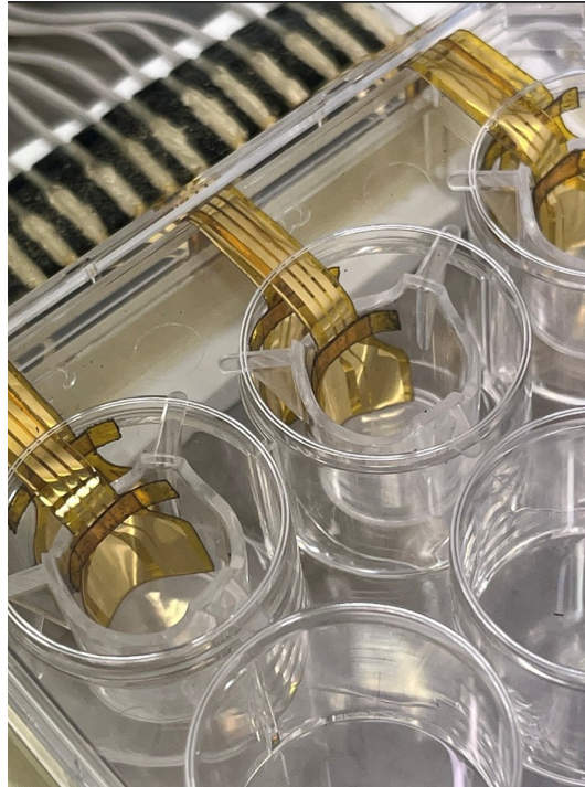
Figure 3.36: Close-up view of the Top and Bottom OECTs integrated in the multiwell plate.
