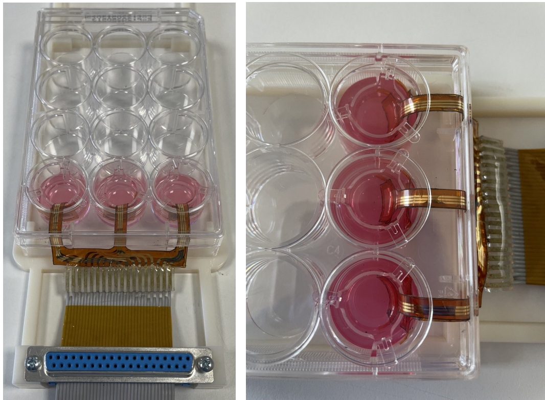
Figure 4.26: Device setup with cell culture medium inserted in the wells and transwell inserts.
