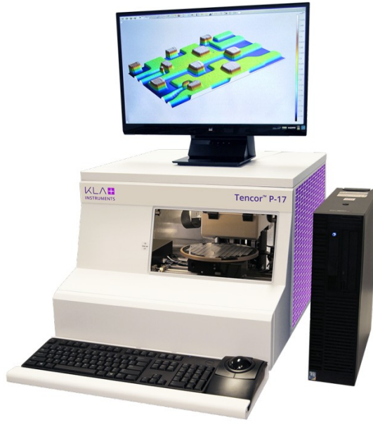
Figure 3.24: Tencor P-17 stylus profiler used for the profilometric analysis.
