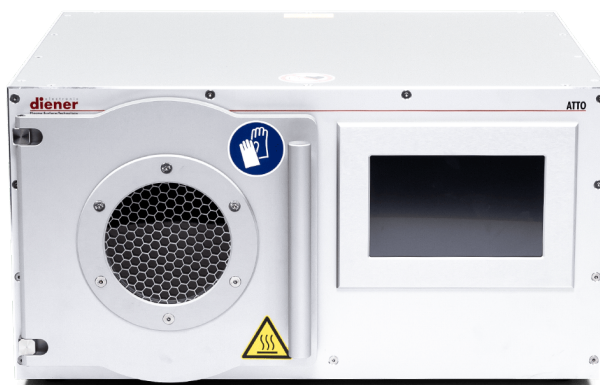
Figure 3.27: Diener Atto plasma system used at ChiLab laboratory to perform oxygen plasma treatment.
