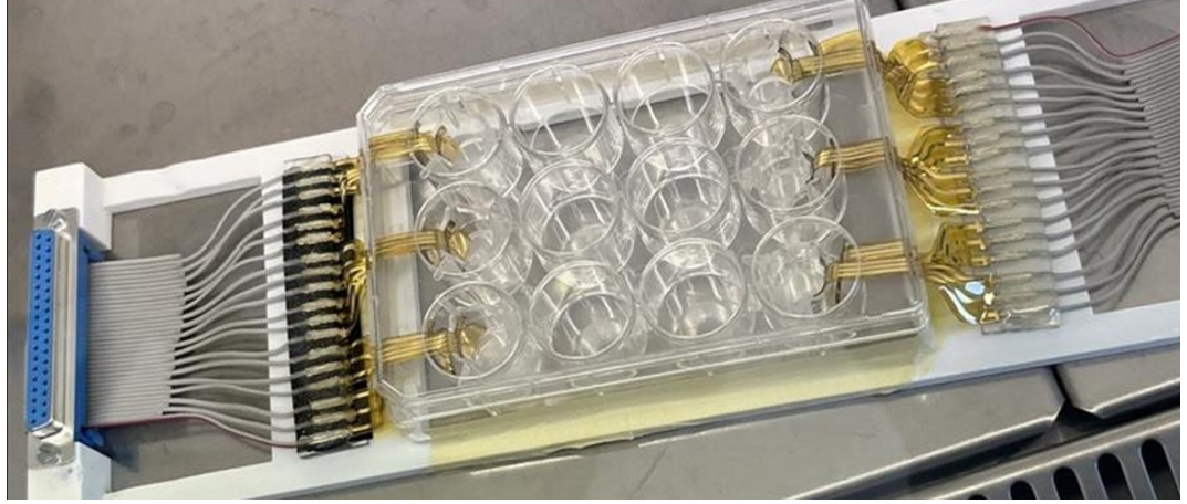
Figure 3.35: Whole setup after sterilisation, before Caco-2 cells are seeded.
