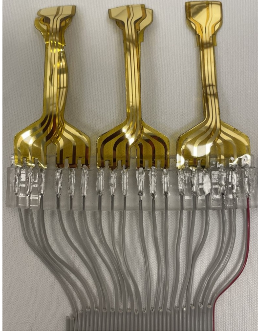
Figure 4.17: Final result of the device once the contacts with the ribbon cable are formed.
