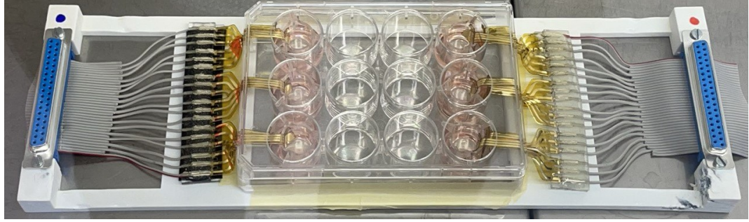
Figure 4.24: View of the alternative design device mounted on the supporting structure. The branches of the structure were made longer to better accommodate the ribbon cable.
