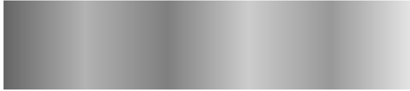
Figure 3.21: 24-bit bitmap pattern for skyrmion "burst" motion. Darker areas correspond to smaller dwell times and light areas to longer dwell times.
