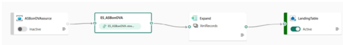
Figura 6.1: Full Eventstream pipeline from ASBonOVASource through transformation and routing into Eventhouse bronze tables.
