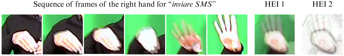
Figure 3.10: Sequence of frames and two resulting HEIs for the right hand performing the sign inviare SMS . HEI 1 is obtained from blurred RGB frames; HEI 2 is constructed from thresholded and then blurred frames.
