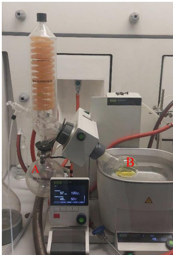
Figure 11 Rotary evaporator; A) Solvent collector flask after its evaporation, B) Original flask
