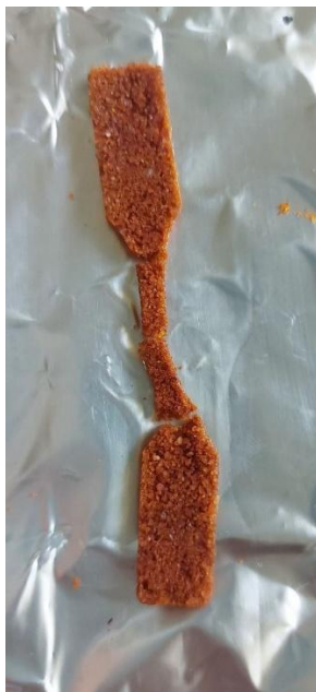
Figure 34 Hot pressed sample in 150°C for 15 minutes
