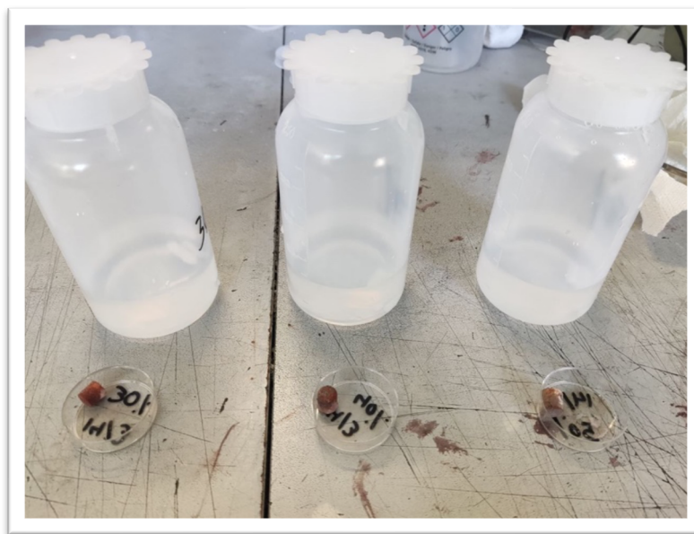
Figure 2-9: Sealed chambers for a humid environment.
