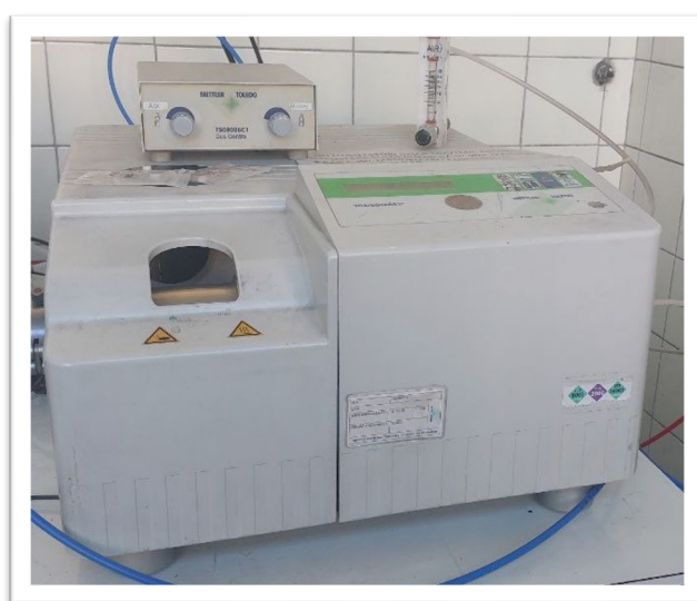
Figure 2-11: Setaram TGA system with a Mettler Toledo TGA/DSC gas control
