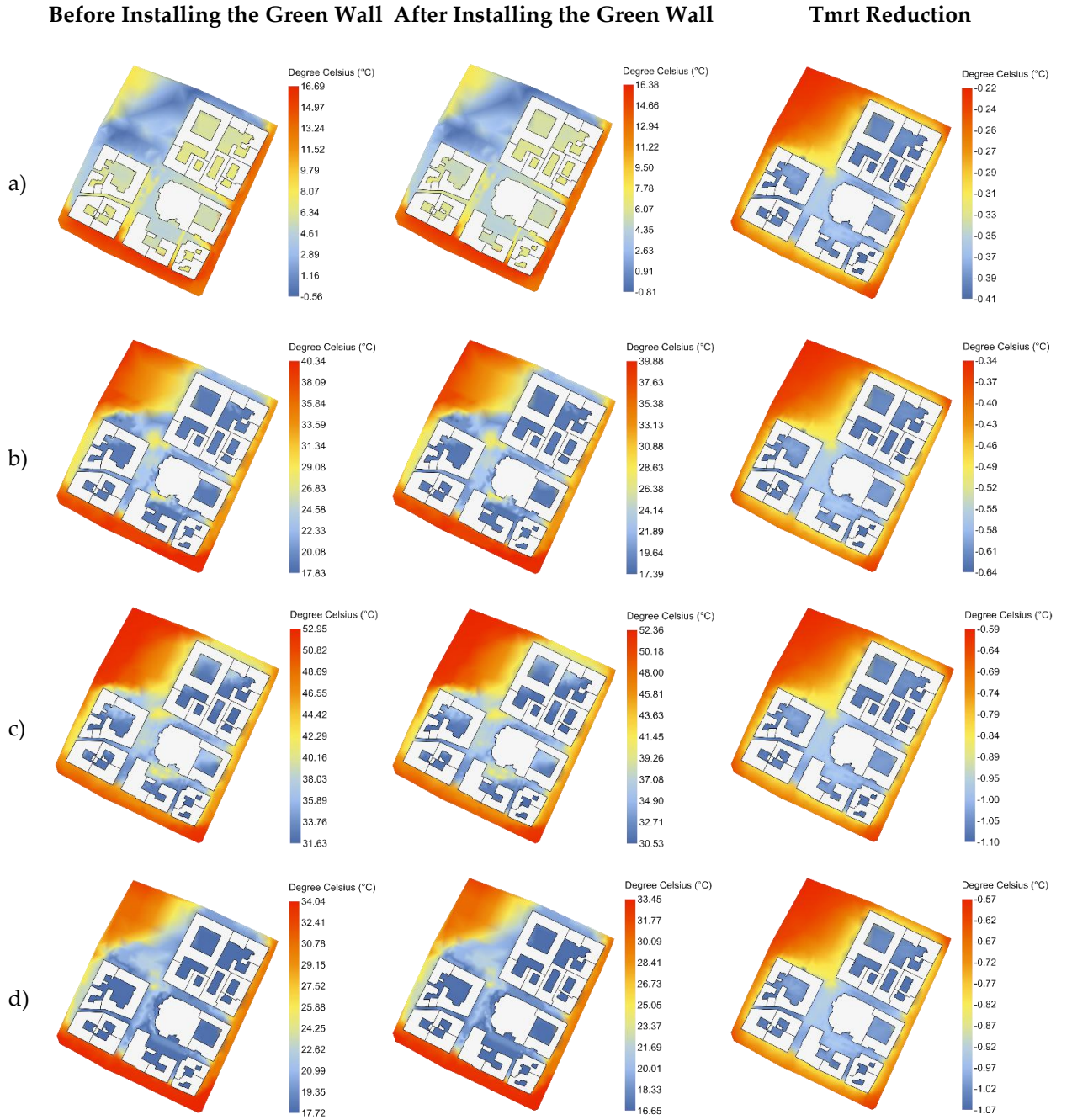
Figure 6. Mean radiant temperature (Tmrt) °C spatial heat map before and after the installation of the green walls and the enhancement effect of green walls under current weather conditions. a) 12 th January; b) 29 th March; c) 29 th July; d) 15 th October.
