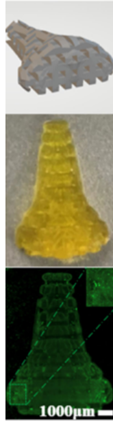
Figure 1.19: 3D-printed nasal hydrogel scaffold (model and optical image) and live-dead staining of cells at Day 7 show cell viability in the printed construct. [70]
