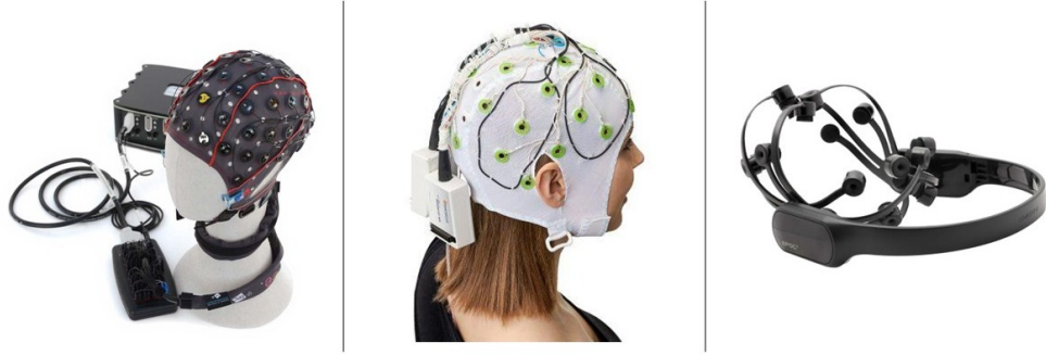
Figure 2.3: Three examples of state-of-the-art EEG devices. From left to right: g.tec g.GAMMAsys with dry electrodes for high-density, quick setup; Brain Products BrainCap featuring active electrodes for high signal quality; the portable Emotiv EPOCH X, ideal for everyday applications.
