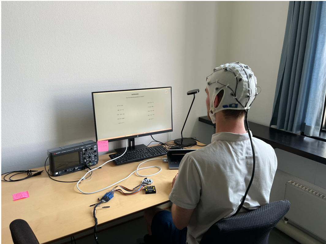
Figure 4.12: Experimental Setup. The subject is positioned in front of the screen with the interfaces. The EEG cap is connected via cables to the amplifier, which is connected via Bluetooth to the USB dongle in the laptop.
