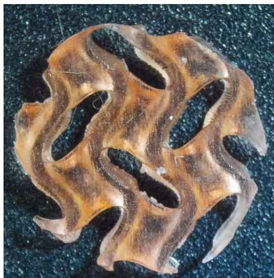
Figure 4.4 Bottom view of a printed NIP. Image obtained with an optical microscope
