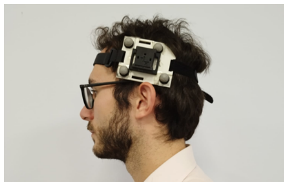
Figure 7.1: Support with INDIP sensor and markers
