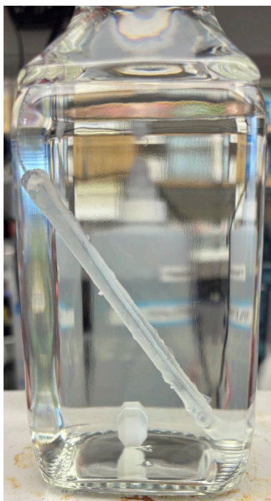
Figure 41. Setup for PTX release from coated balloon.
