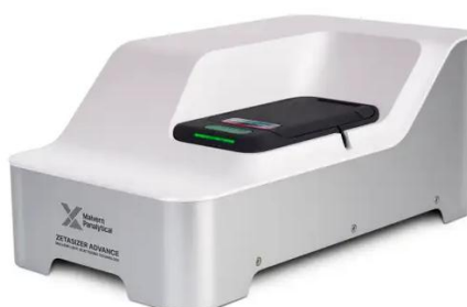
Figure 9: Picture of the used Dynamic Light Scattering device (DLS) ZETASIZER ADVANCE PRO, software ZS Xplorer, Malvern Panalytical) 60
