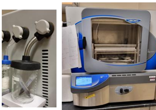
Figure 7: Picture of the used Freeze-dryer machine (FreeZone Triad Freeze Dryer, Labconco Corporation, Kansas City, MO, USA)
