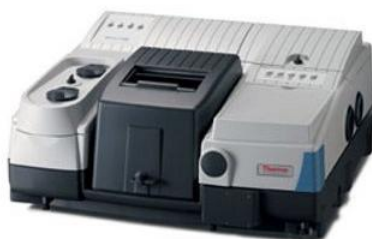
Figure 13: Picture of the used Fourier Transform Infrared Spectrometer (FT-IR) (Nicolet 6700, Thermo Fisher Scientific, Waltham, Massachusetts, USA) 67 .
