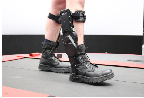
Figure 3.7: Active Dephy ExoBoot (EB60) by Dephy Inc. [24].
