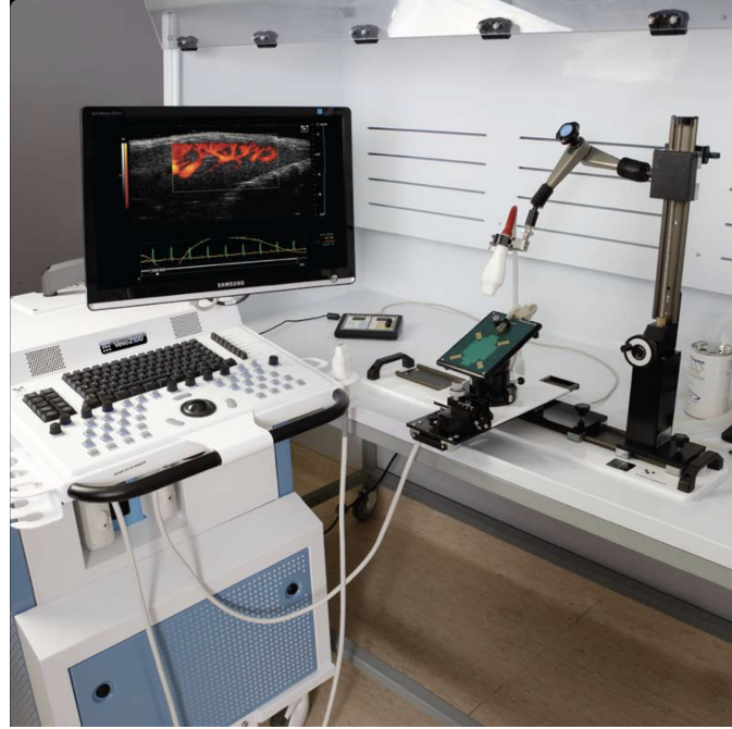
Figure 2.5: Vevo 2100 Ultrasound Imaging System (FujiFilm VisualSonics Inc., Toronto Canada) [32, 85]. The Vevo 2100 Imaging Platform - featuring high-frequency, high-resolution ultrasound with linear array technology and Color Doppler - delivers 30-micron resolution, frame rates up to 1000 fps, and advanced 3D imaging for preclinical research across multiple animal models and disciplines.
