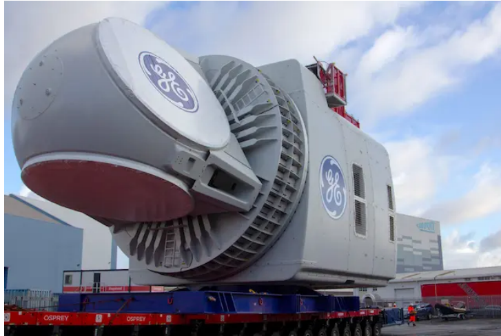
Figure 1.7: GE's Haliade-X 12 MW nacelle
