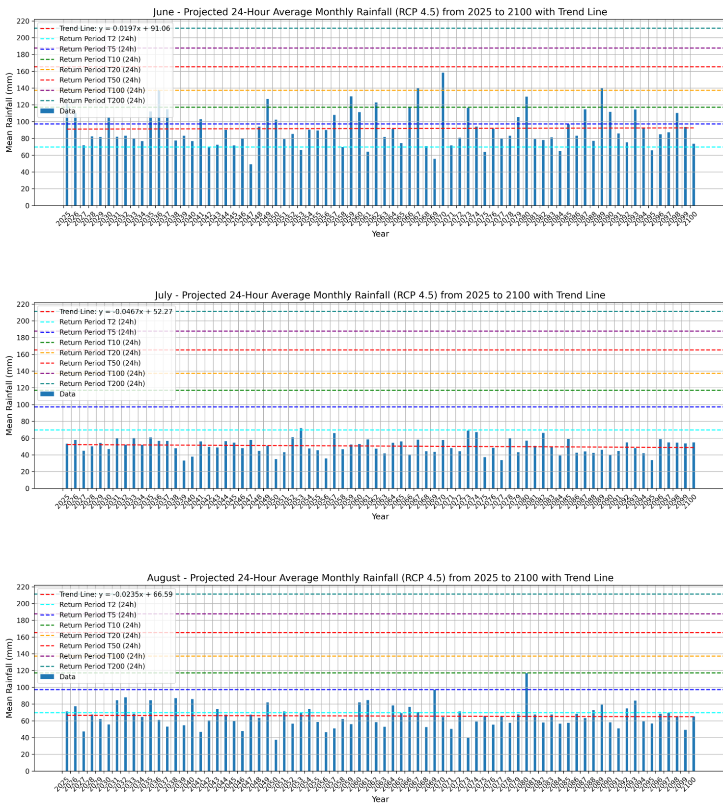
Figure 76_Return Period of Cumulative Rainfall per 24 hours with Trend Line from 2025 to 2100, RCP 4.5_ Jun to Aug
