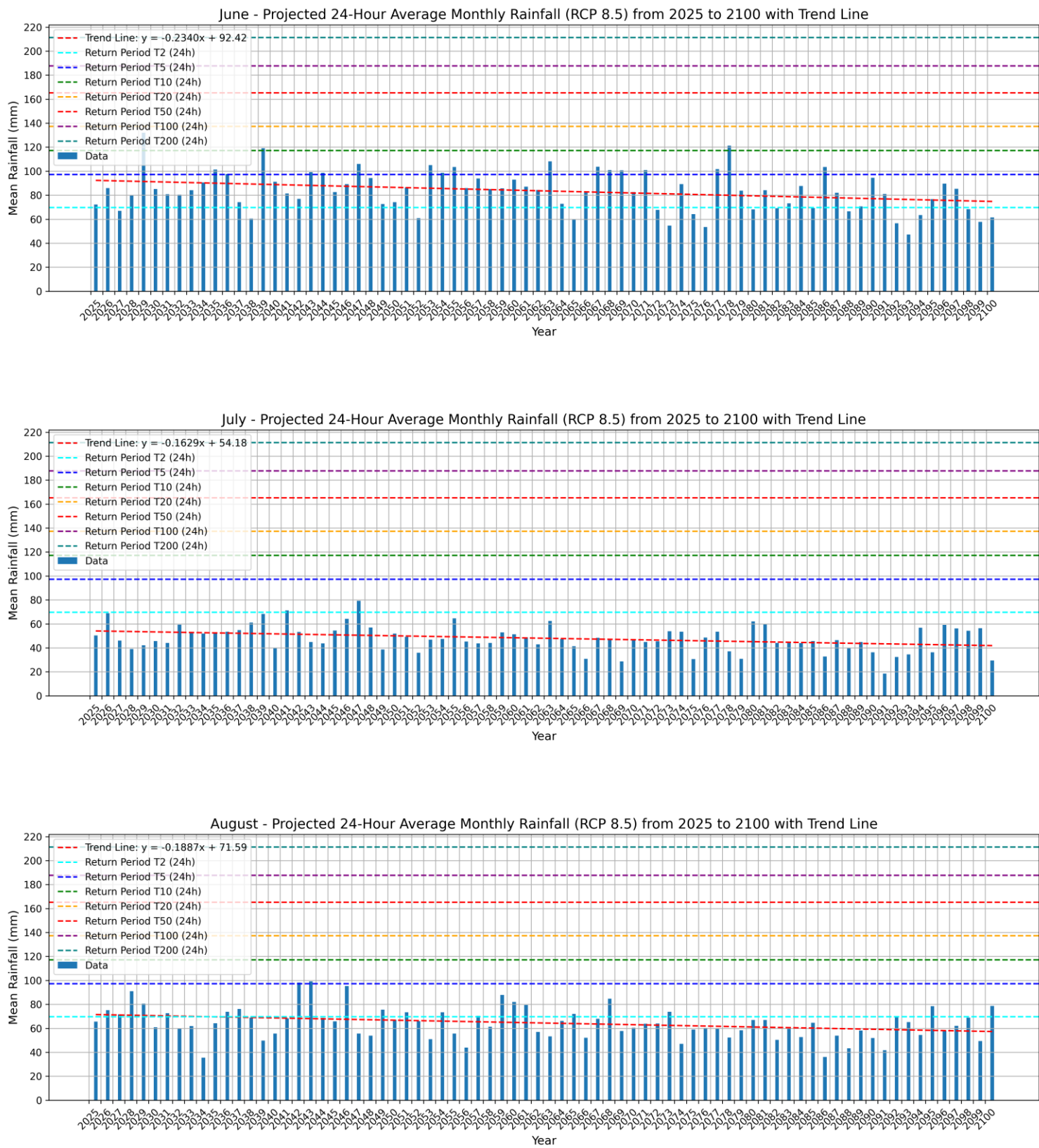
Figure 108_ Return Period of Cumulative Rainfall per 24 hours with Trend Line from 2025 to 2100, RCP 8.5_ Jun to Aug
