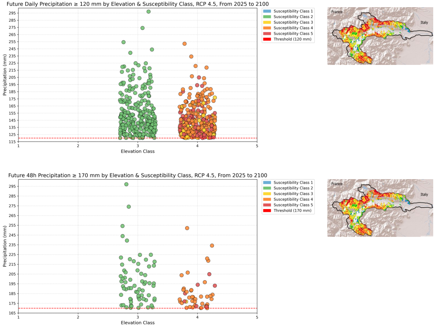
Figure 82_ 24 and 48 hours Rainfall Events by Elevation Class and Rockfall Susceptibility, RCP 4.5
