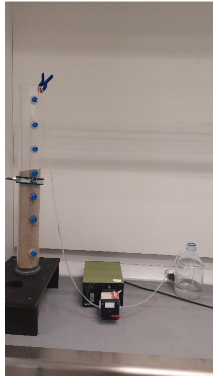
Figure D.6 Saturating the column from the top with tap water through a peristaltic pump
