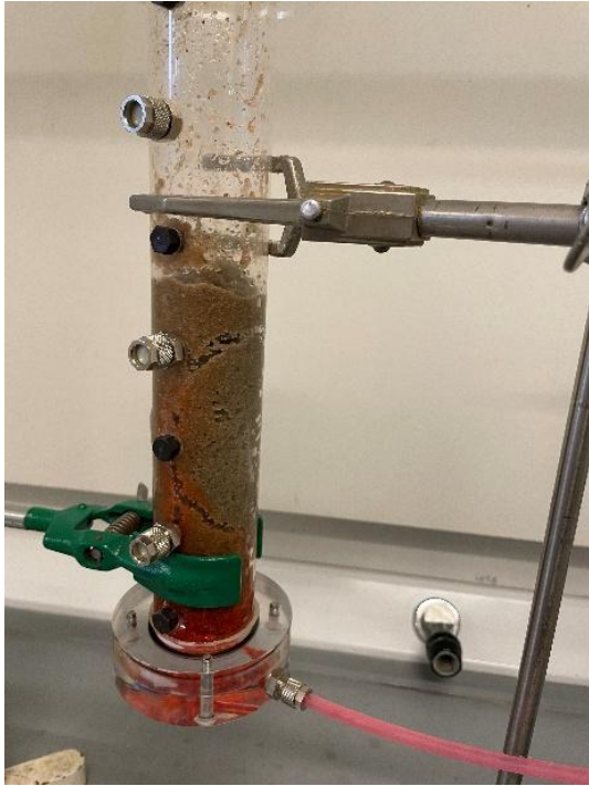
Figure A.5 Fractures in the column caused by too high air flowrate. Test nr.2 on date 28/02/25.
