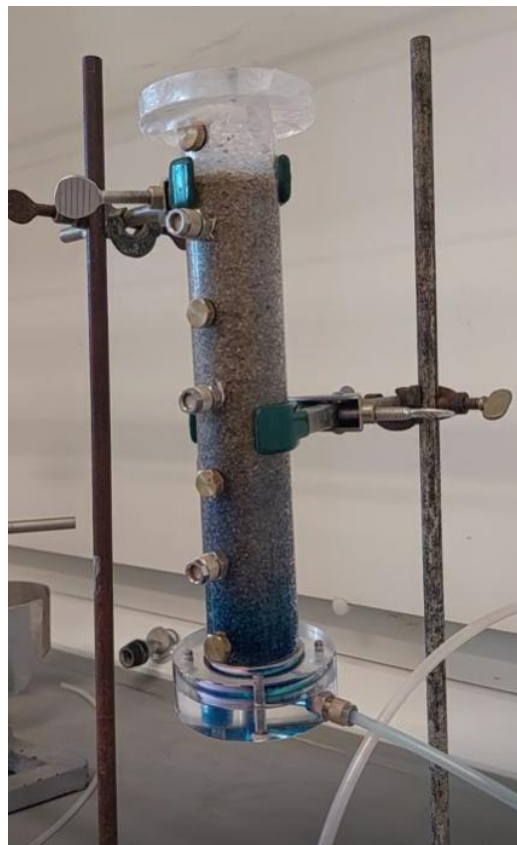
Figure A.7 Persil detergent mostly concentrated at the bottom of the column because too dense. Certain migration of the detergent attached to air bubbles. No migration of Methylene blue showing no advective water flux. Test nr.8 on date 25/03/25.
