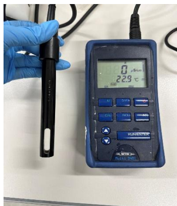
Figure 10 (a) EC meter (MULTI340i with Tetracon 325 probe) (b) PH meter (XS pH 70 Vio, XS Instruments)
