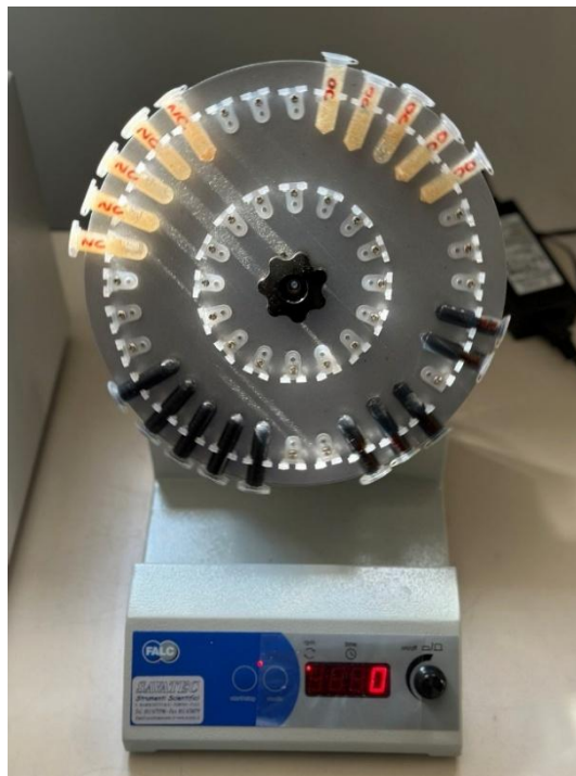
Figure 12 The overhead shaker used during the batch adsorption tests for sample mixing
