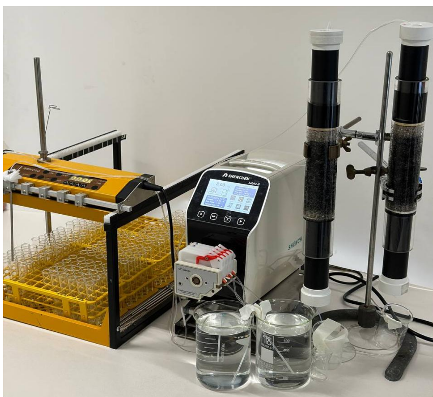
Figure 14 column transport test setup
