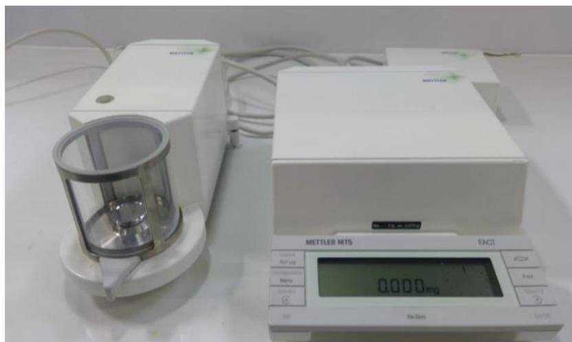
**Figura 3.9:** Micro bilancia Mettler Toledo MT5
