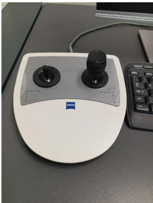
**Figura 4.19:** *SEM Dual Joystick*
