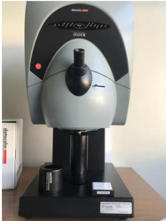
**Figura 4.7:** Datacolor Spectroflash SF 600X
