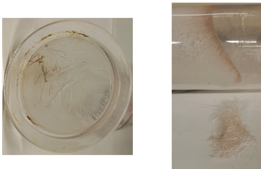
Figure 22: Needle-like crystals formed in the tube during the pyrolysis of MA010.
