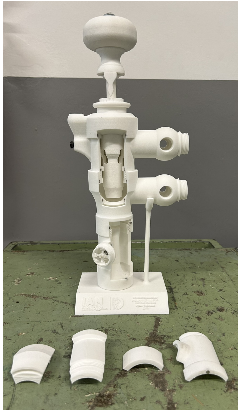
Fig. 5.18 Final polymer prototype with sections opened
