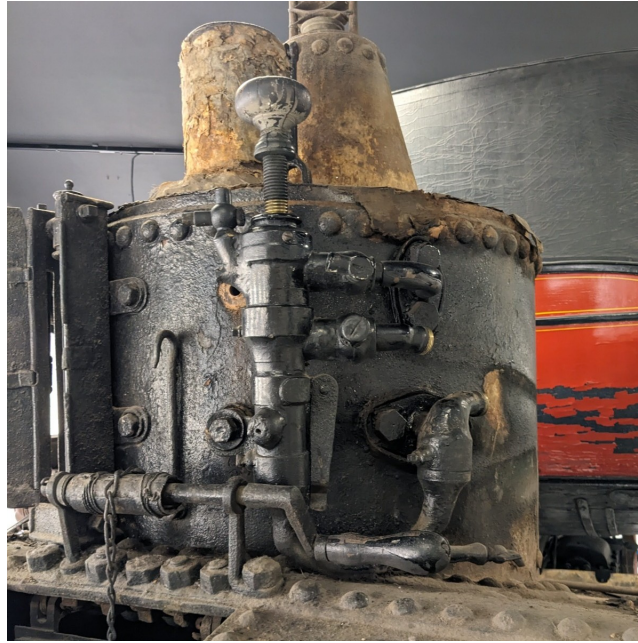
Fig. 5.6 Bordino injector mounted on the boiler
