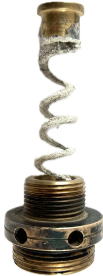
Fig. A.21 Upper stuffing box. The white spiral is the stuffing.
