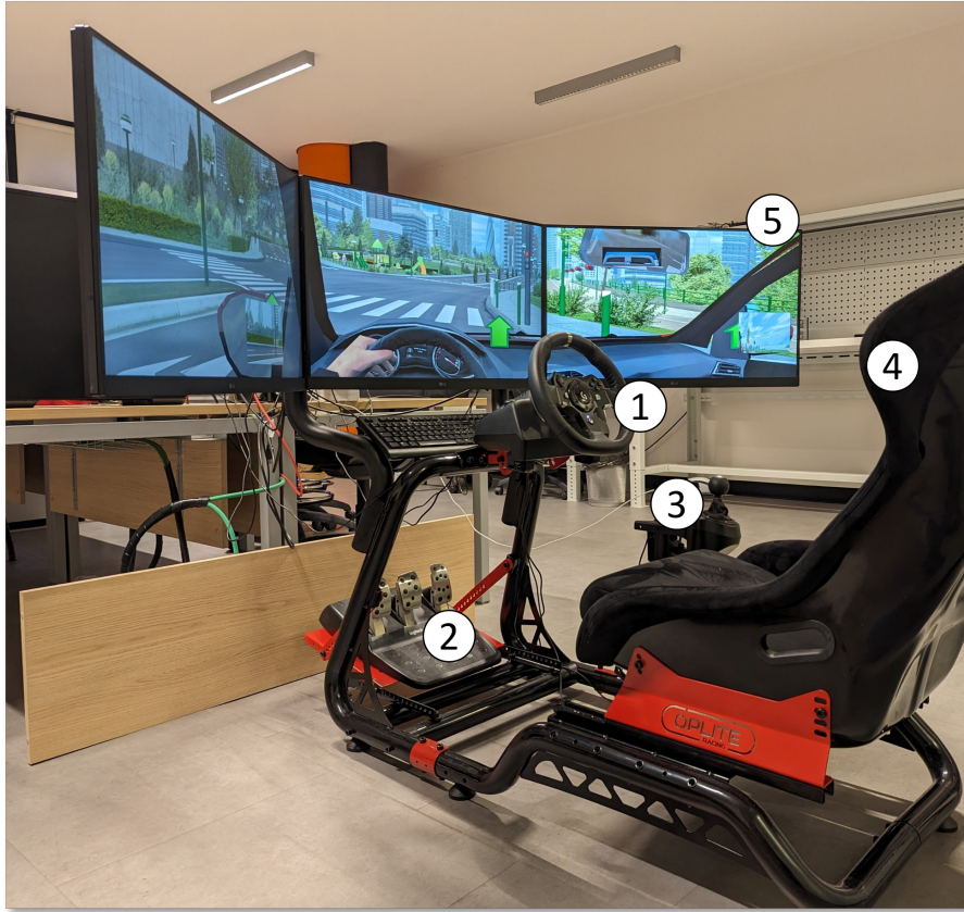
Figure 2.4: Driving simulator paired with SCANeR™ Studio. 1: force feedback steering wheel, 2: pedals, 3: manual gearbox, 4: bucket seat, 5: high resolution screens.
